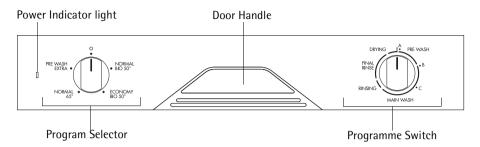
Set the point at which the wash programme is to start using the **programme switch**. The programme switch rotates during the wash programme and indicates the position that has been reached in the programme.
